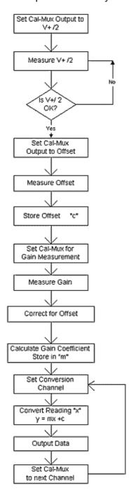
Figure 2. This flow chart details a calibration procedure implemented in the Figure 1 system.
